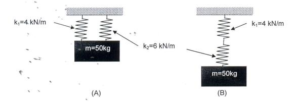
Figure 2: Spring arrangement
