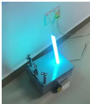
Fig. 5. Testing of UV Sanitiser prototype
