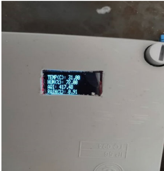
Fig. 29.6 Information data display on OLED
