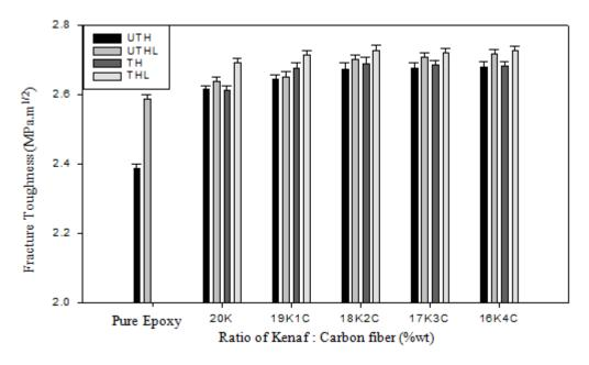
Figure 3 Fracture taughness of epoxy reinforced hybrid kenaf/carbon fiber composite
