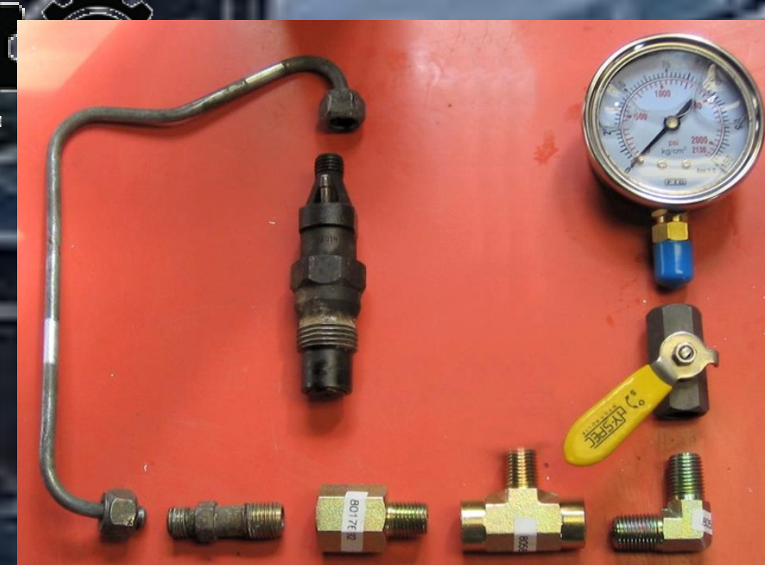
Fig. 3 : Arrangement from various components to create the pressure tester
