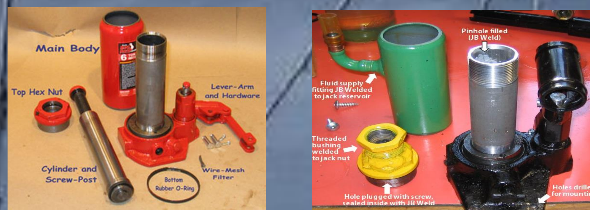
Fig. 2: Components of the HYDRAULIC JACK
