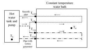
Fig. 4: Apparatus to determine heat transfer coefficient. Black dots indicate the location of Type K thermocouples and the arrows show the direction of fluid flow.
