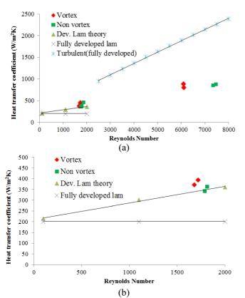
Figure 6: (a) The comparison of heat transfer coefficient between the theoretical, pipe with vortex and smooth pipe, and (b) Enlarged view of laminar flow region.
