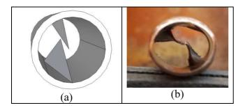
Fig. 3: (a) Schematic of vortex generator and (b) the actual vortex generator inside a 12 mm diameter copper pipe
