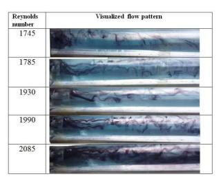
Fig. 5: Flow pattern at various Reynolds number. The inner diameter of the pipe is 12 mm
