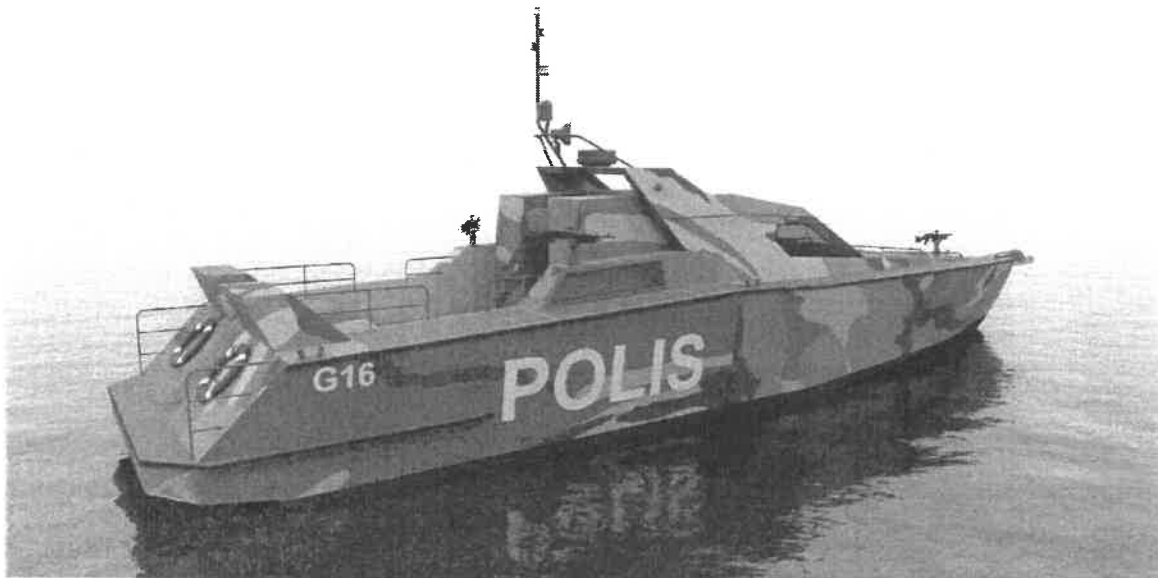
Figure 1.1 A 25 meter waterjet propelled fast attack gun boat designed for Polis Diraja Malaysia (PDRM) to have a sprint speed of 51.6 knots. This design was based on 17.6m LOMOcean design.
