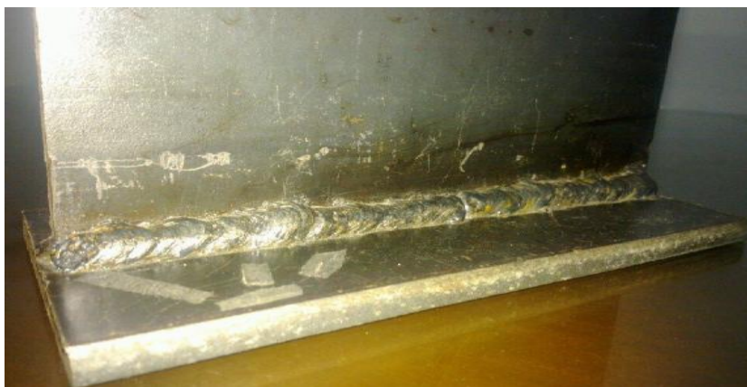
Photo 1 – Tee Fillet Joint
