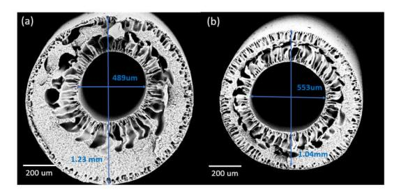
**Figure 5.** The overall (×100 magnification) structure of DLHF membranes spun at air gap of 5 cm for (a) DL-ZT0 and (b) DL-ZT1.
