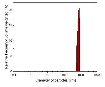
Figure 4. Distribution of ZrO<sub>2</sub>-TiO<sub>2</sub> nanoparticles
