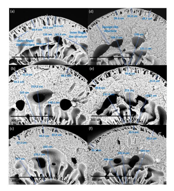
**Figure 7.** The cross-section (×300 magnification) structure of DL-ZT1 membranes spun at different air gap of (**a**) 5 cm, (**b**) 10 cm, (**c**) 20 cm, (**d**) 30 cm, (**e**) 40 cm, and (**f**) 50 cm.
