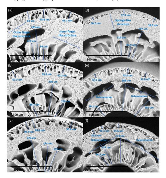
**Figure 6.** The cross-section (×300 magnification) structure of DL-ZT0 membranes spun at different air gap of (**a**) 5 cm, (**b**) 10 cm, (**c**) 20 cm, (**d**) 30 cm, (**e**) 40 cm, and (**f**) 50 cm.
