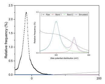
Figure 2. Zeta potential of ZrO<sub>2</sub>-TiO<sub>2</sub> nanoparticles with inset showing the deconvolution of two peaks.
