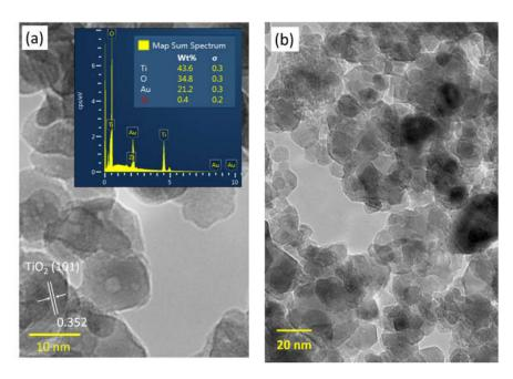
**Figure 3.** Transmission electron microscopy (TEM) images of  $ZrO_2$ -Ti $O_2$  nanoparticles. (a) Ti $O_2$  crystal spacing with inset shows the peaks and the percentage of elemental composition and (b) Small agglomeration and dispersion of nanoparticles.
