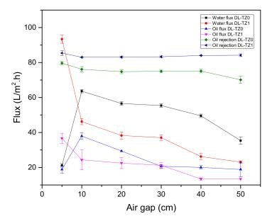
Figure 10. Effect of air gap on flux and oil rejection.
