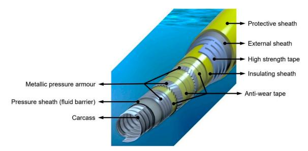
Figure 1. Schematic of a typical flexible umbilical cable for offshore engineering.
