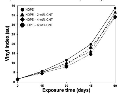
**Figure 7.** Vinyl indices ( $I_{CO}$ ) of the monolithic and nanocomposite films exposed to UV-B radiation.
