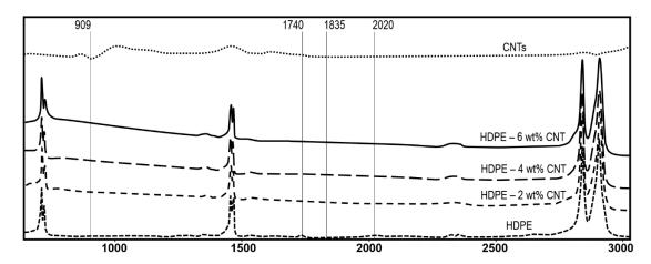
Figure 5. IR spectrum of HDPE, CNTs and nanocomposite films without exposure to UV radiation.
