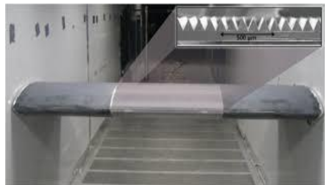
Fig. 1 Riblets on a wing
