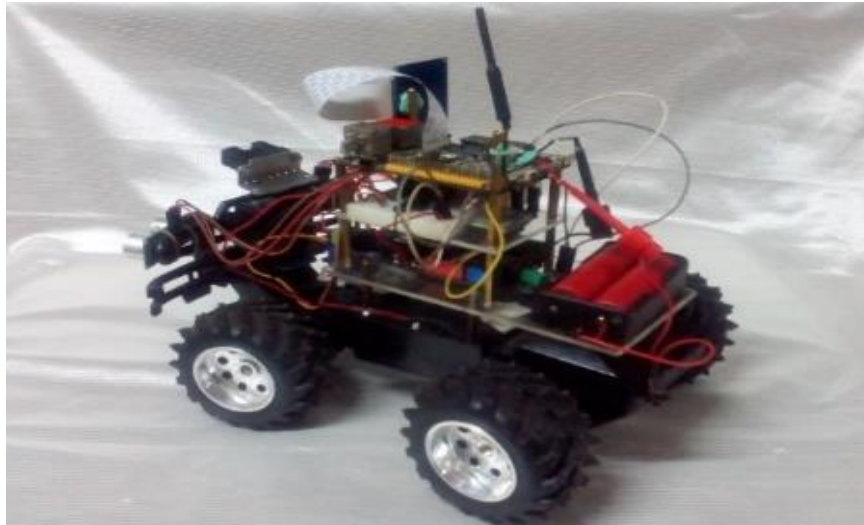
Figure 5. ToMRobot Components for MANET Testbed (Actual Implementation)
