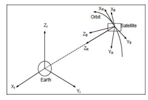
Figure 1 Definition of the orbit reference frame [1]
