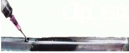
Fig. 2: Dye injection method to make the flow pattern visible
