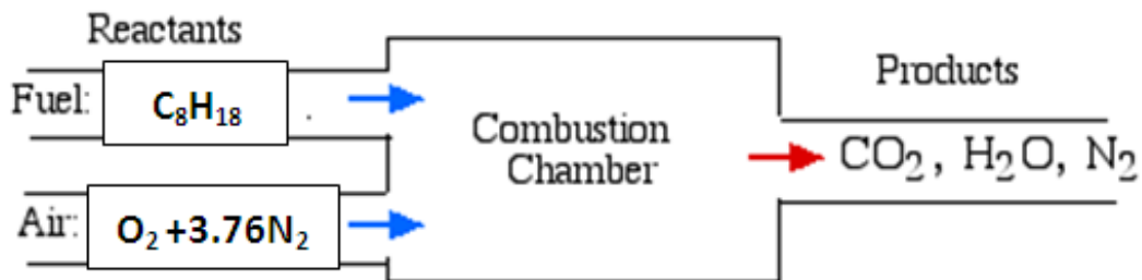
Figure 2: The combustion process layout of internal combustion engine (Spark Ignition engine)
