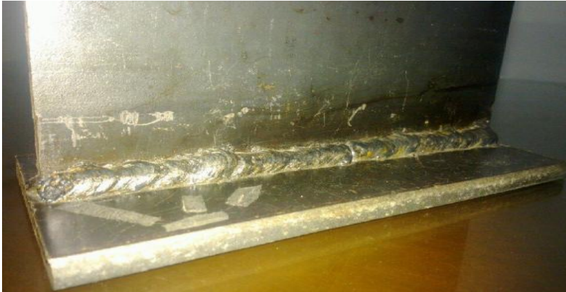
Photo 1 – Tee Fillet Joint
