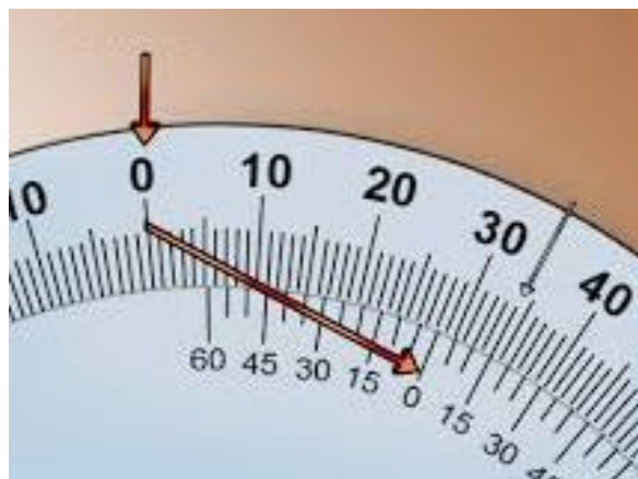
Figure 3: Universal Bevel Protractor
