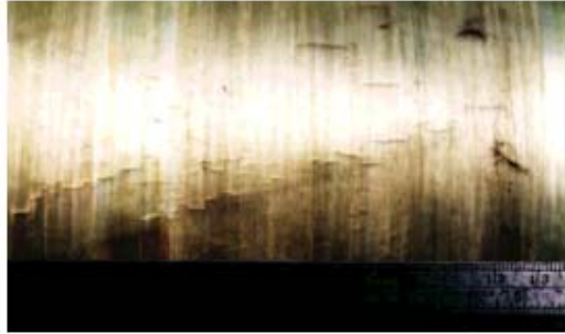
Figure 2: Stress Corrosion Cracking (SCC)
