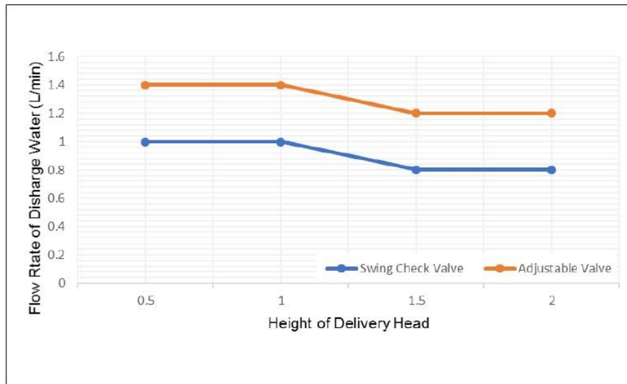
Figure 8. Comparison of swing waste valve and adjustable waste valve
