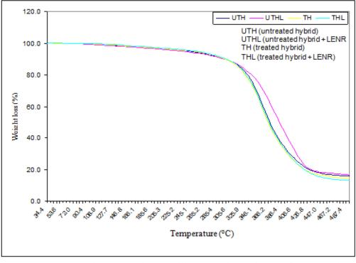
Figure 2 Comparison of TGA curve of epoxy reinforced hybrid kenaf/carbon fibre composite
