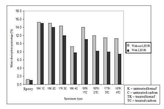
Figure 1 Water absorption percentage of epoxy reinforced hybrid kenaf/carbon fiber composite with and without LENR after 120 days.
